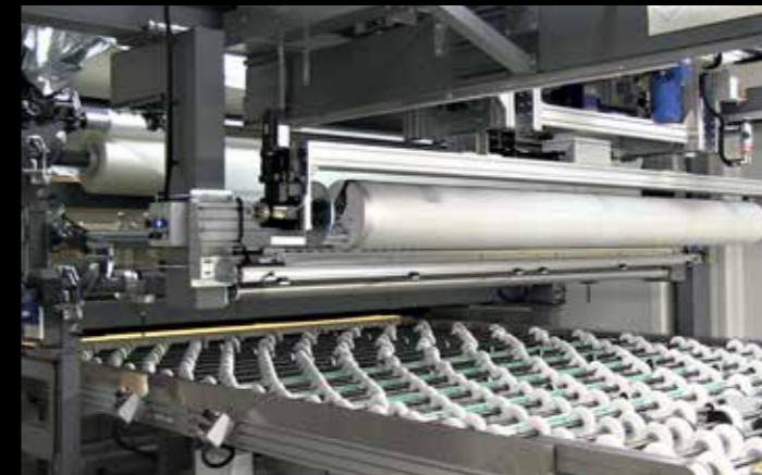
PVB rolls magazine and in-line cutting Configurable with 3 / 6 / 8 roll holders; the roll is installed and unwound automatically. Roll rotation is driven by a gearmotor. Includes the gripper to pick up the PVB and automatic cutting on the X axis.
