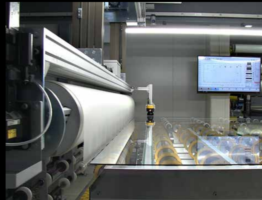
PACMAN automatic cutting and laying system Our PACMAN automatic cutting and laying system automatically picks up the PVB from the rolls magazine and cuts it to the required size. The PVB sheet is then picked up by the PACMAN and spread automatically and accurately on the glass, without requiring any operator action. If necessary, the PVB can be laid ready-cut to the required size manually without difficulty, thanks also to optimal accessibility to the laying zone.
