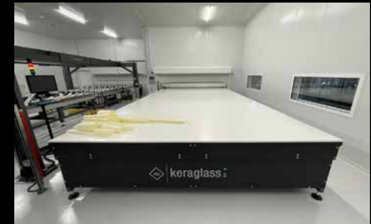
PVB cutting table (off line) Composed of a rotary rolls magazine configurable for up to 8 rolls, the table picks up the required length of PVB by means of an automatic gripper. This system is designed to allow advance preparation of PVB sheets cut to measure to offer the maximum production flexibility.
