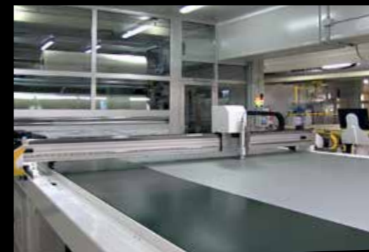
Automatic cutting table The innovative automatic cutting table makes it possible to prepare the PVB quickly, also for shaped cuts. The table transports the PVB by means of a special belt that guarantees low friction movement without damaging the film thanks to an air cushion, and simultaneously assures precise positioning at the time of cutting. Computer controlled axis movements mean that any shape can be cut with extreme precision and repeatability to give savings in production times. This system is ideal when the size of the sheets to be coupled changes constantly using a dedicated cutting optimisation software application.
