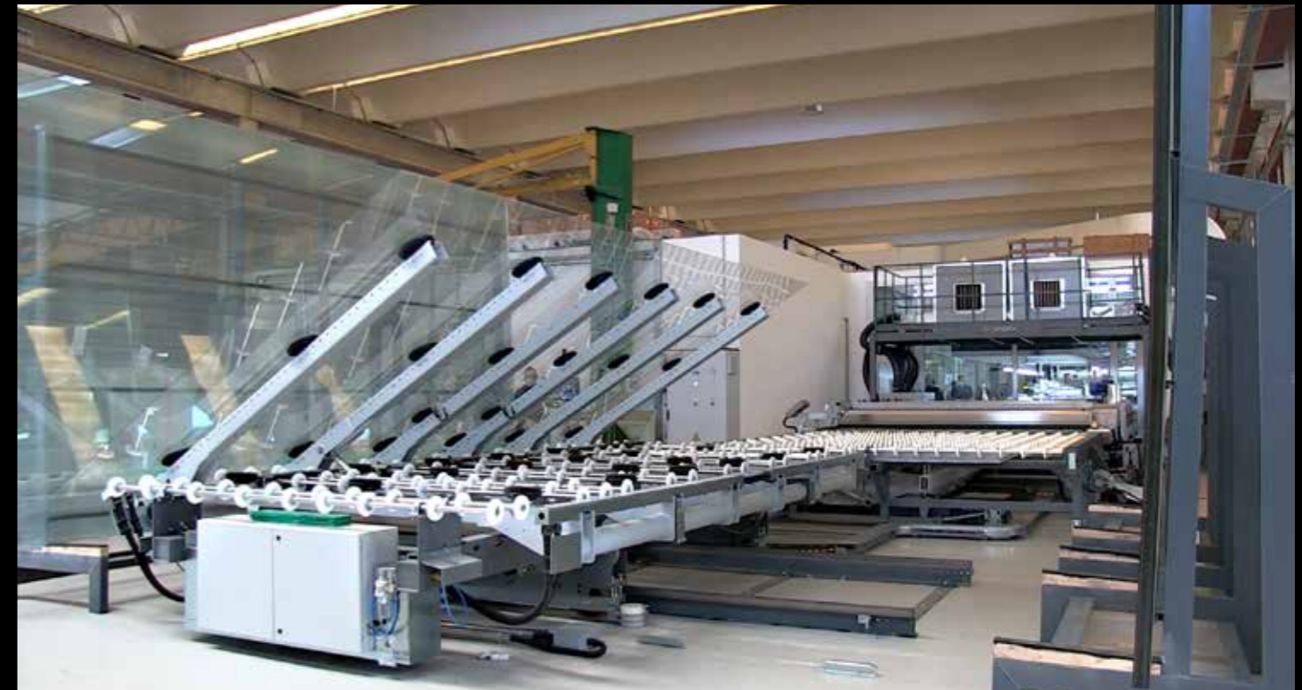
Single side automatic loader for large sheets
