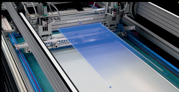
STAGE 3 Enamel flooding on screen
