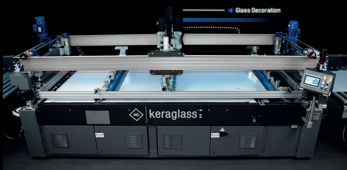
STAGE 4 Enamel transfer onto panel
